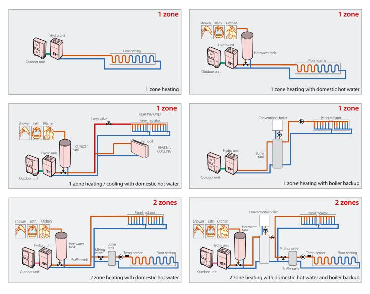
In existing dwellings already equipped with traditional gas or fuel boilers, Toshiba Estía air to water heat pump system can be combined with the existing heating system to cover exclusively and in an optimized way all the heating needs, all year round. Then, the boiler is only used as a back-up source during some extreme weather days of the winter. The intelligent Toshiba control balances the energy source in the most efficient way.
